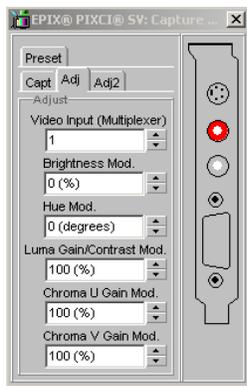
The XCAP imaging program features a Capture & Adjust Dialog dedicated to controlling the PIXCI SV5 imaging board.
