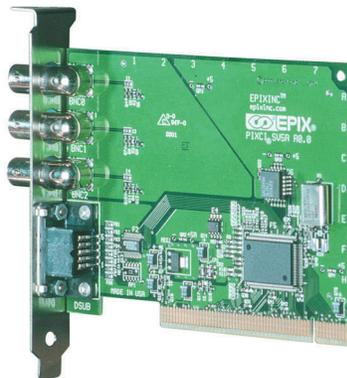
The PIXCI SV5A offers 3 BNC connectors instead of 2 BNC and 1 S-Video — all other features are identical to the PIXCI SV5.
